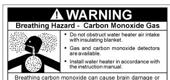
• Do not apply insulation to the top of the water heater, as this will interfere with safe operation of the blower assembly.
